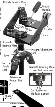
**Telescope Attachment Diagram**
